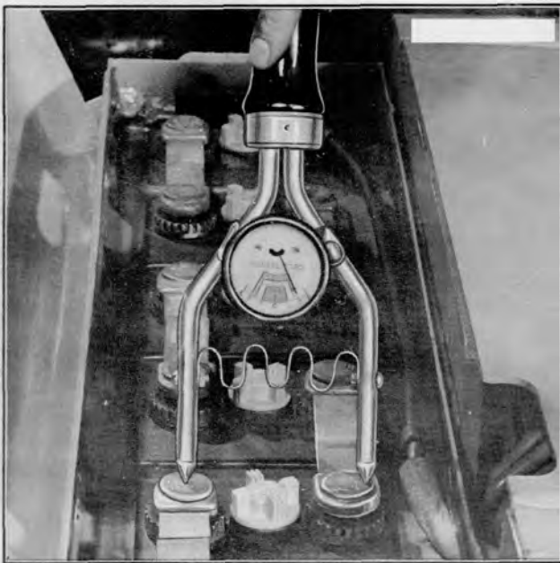
Plate 4008. Charge Test Fork Check
