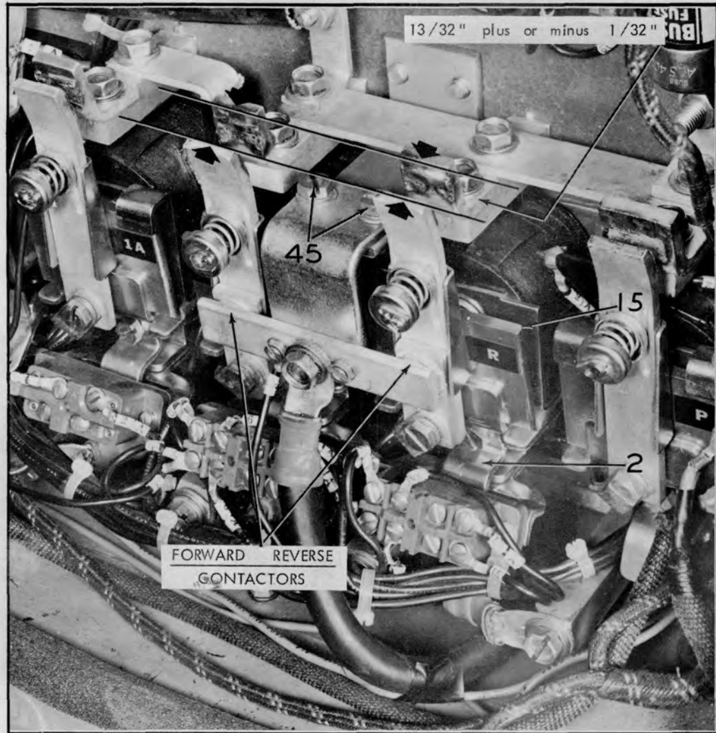
Plate 6599. Forward and Reverse Contactor Checks
