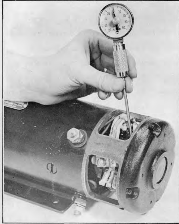
Plate 6560. Typical Method Checking Brush Spring Tension
