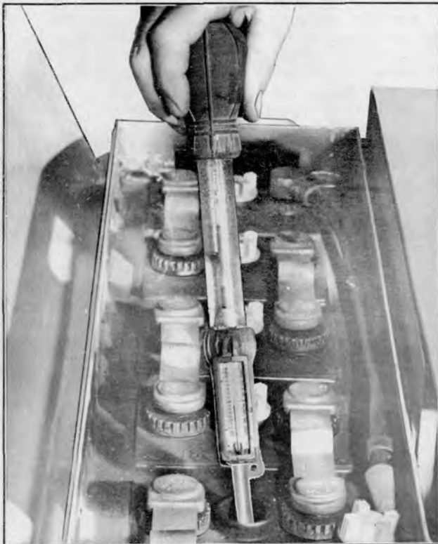
Plate 4018. Hydrometer Check Method
