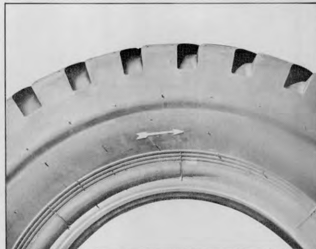
Plate 6422. Inside Dual Tire (or Single Drive Tire) (Arrow to point toward front of truck)
