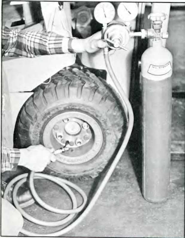
#11500. Clip-on Air Chuck & Nitrogen Cylinder
