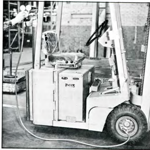
#11501. Shows Set-up Using Nitrogen Cylinder
