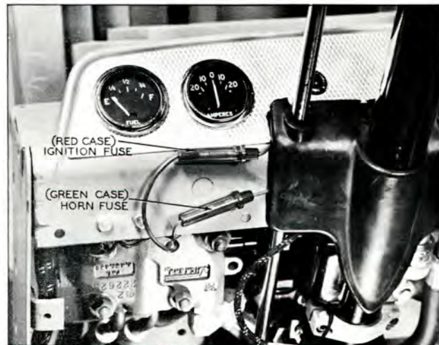
Figure 002b. Ignition Fuse and Horn Fuse
