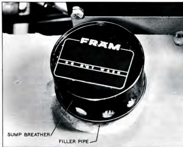
Plate 6626. Hydraulic Sump Tank and Sump Breather
