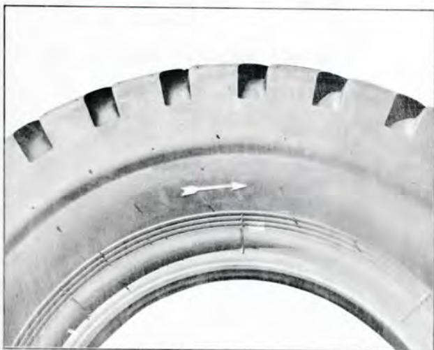
Plate 6422. Inside Dual Tire (or Single Drive Tire) (Arrow to point toward front of truck)
