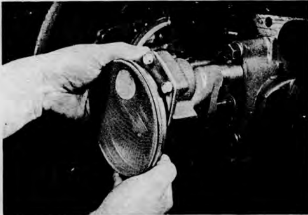
Figure 67 — Oil Pump Removal
