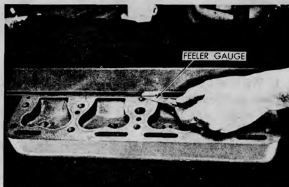
Figure 13 — Checking cylinder head flatness lengthwise.
