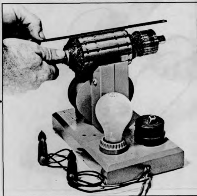
Plate 6996. Checking Armature For Short Circuit
