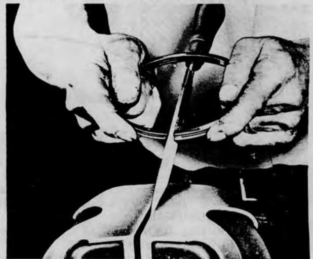
Figure 41 — Filing piston ring to increase gap
