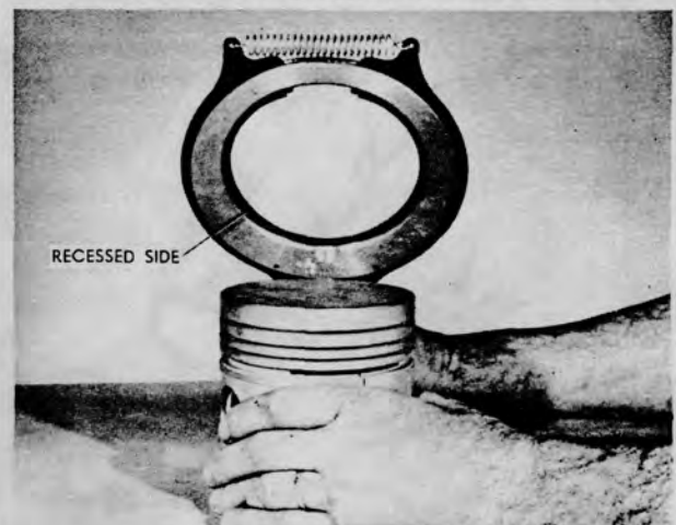
Figure 42 — Installing Rings with Ring Expander Tool
