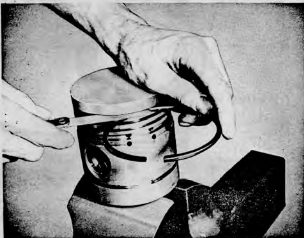
Figure 41 — Checking Ring Clearance in Groove
