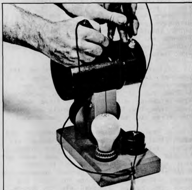
Plate 7223. Testing Field Circuit for Ground
