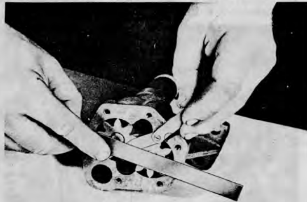
Figure 69 — Checking Oil Pump End Clearance
