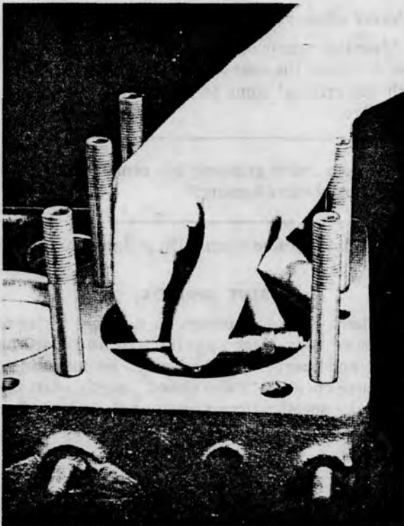
Figure 29 — Measuring original bore diameter above ring travel
