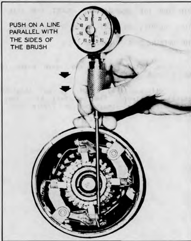
Plate 6449 Checking Brush Spring Tension
