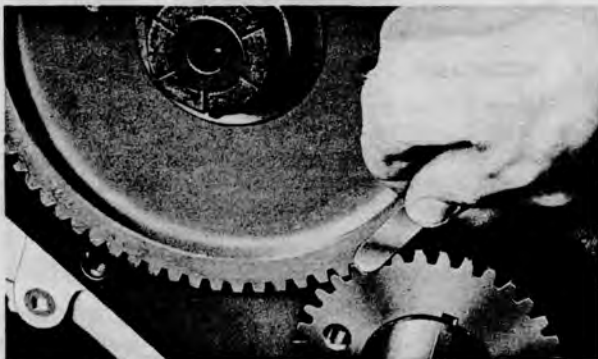
Figure 55 — Checking Timing Gear Backlash
