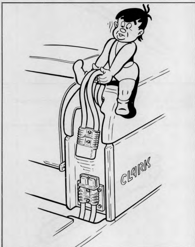
Plate 9688. "Typical" Battery Disconnect
