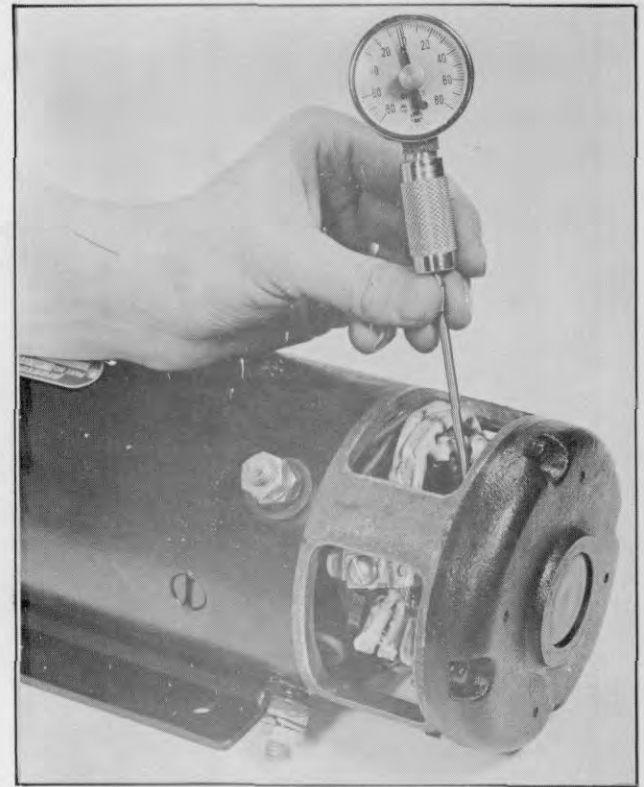
Plate 6560. Typical Method Checking Brush Spring Tension
