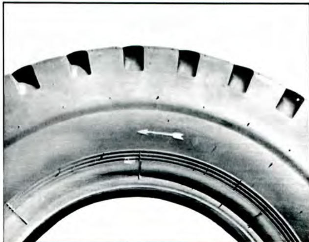
Plate 6423. Outside Dual Tire (Arrow to point toward rear of truck)
