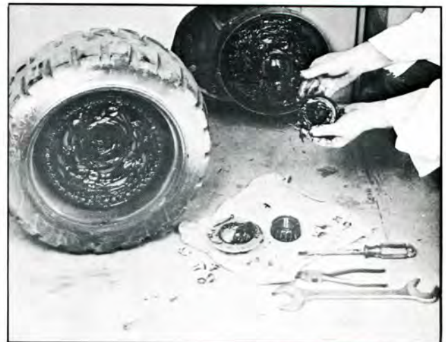
Plate 9775. Repack Axle End
