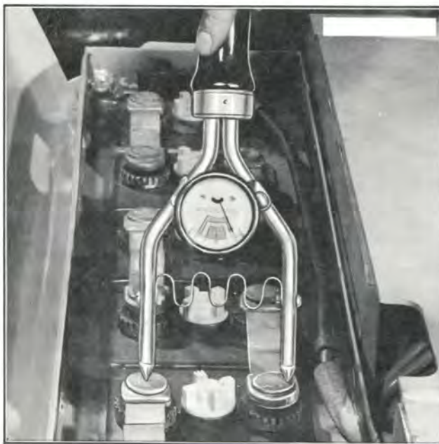
Plate 4008. Charge Test Fork Check
