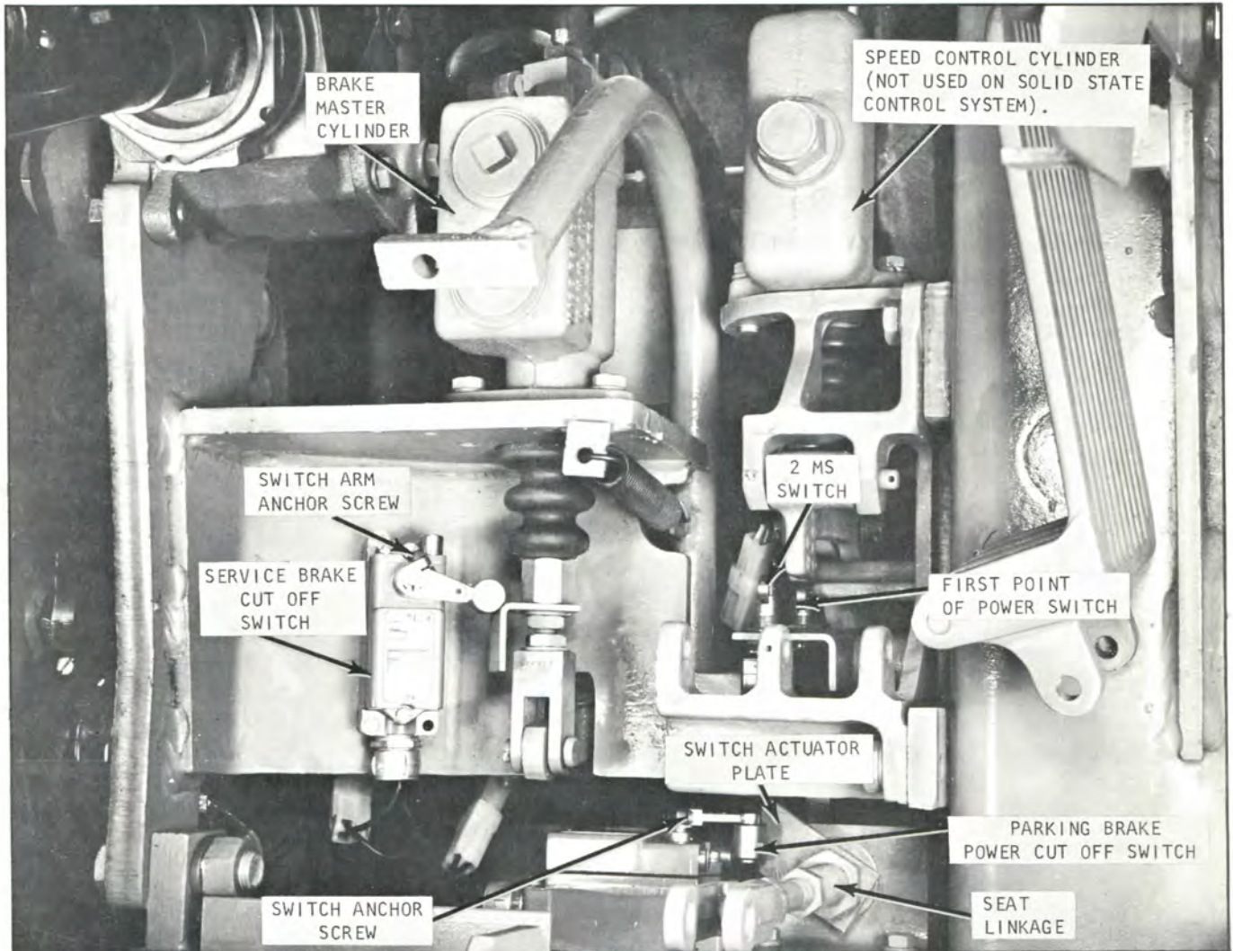
Plate 7545. Parking Brake (Deadman) Power Cut Off Switch; Service Brake Power Cut Off Switch Assy's.
