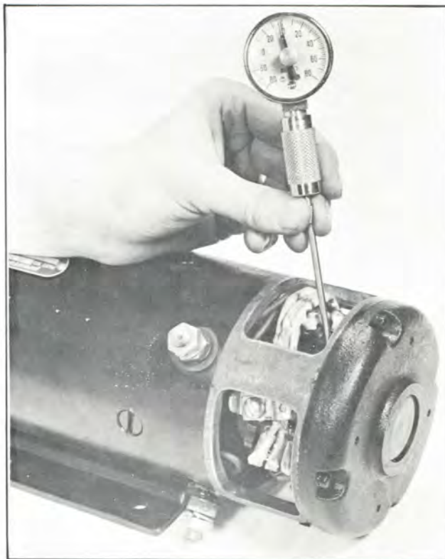
Plate 6560. Typical Method Checking Brush Spring Tension
