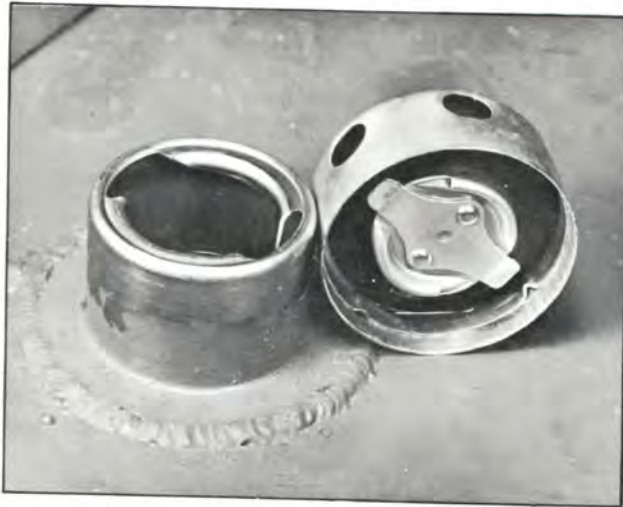
Plate 7046. Typical Hydraulic Sump Tank and Sump Breather
