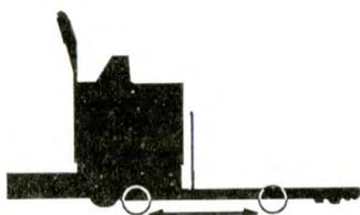
Positioning of forks for lifting AGV.
